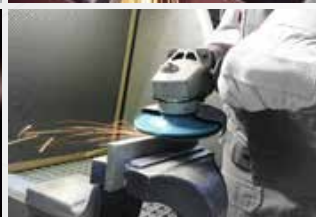
Weld seam preparation
