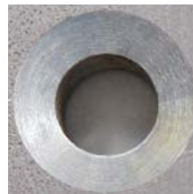
Countersink with extremely unequal spacing
