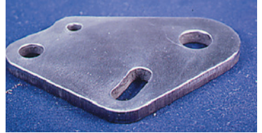
Blanked steel part after deburring.
