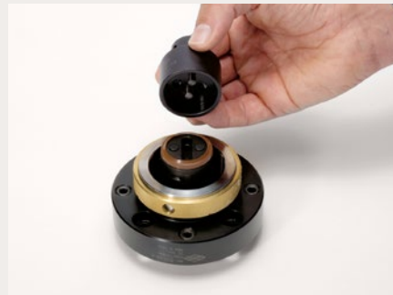
2. Fit socket to the clamping cartridge.
