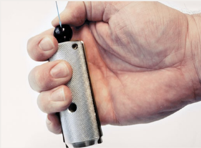
Opening the KS assembly tool
