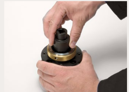
3. Turn clockwise until the lug on the clamping cartridge engages with the clamping pin.
