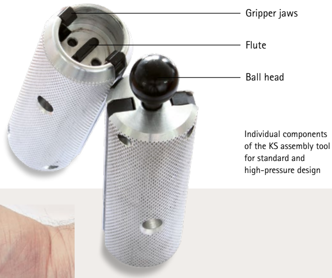
Designation of the individual components of the KS assembly tool
