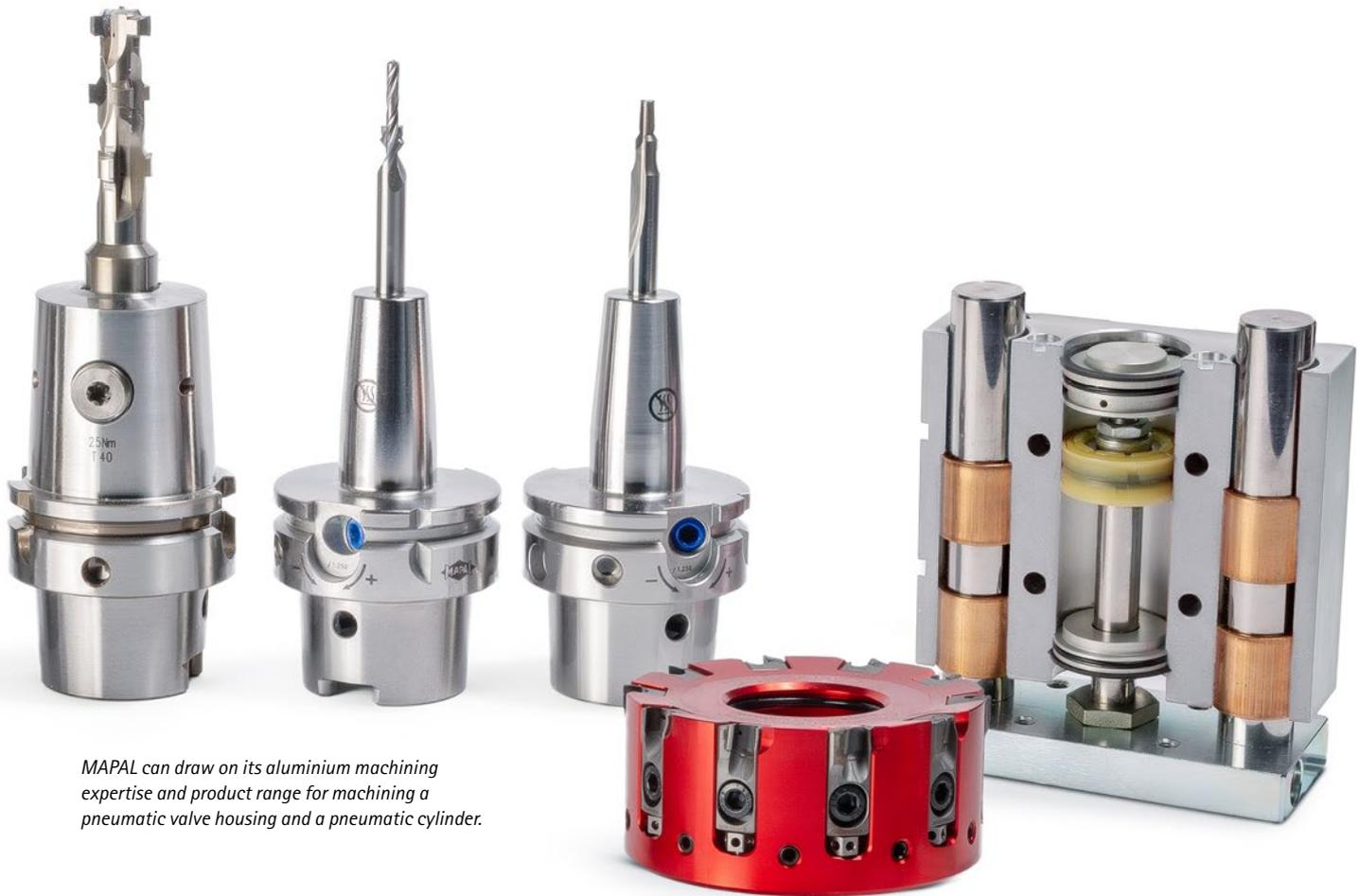
*MAPAL can draw on its aluminium machining expertise and product range for machining a pneumatic valve housing and a pneumatic cylinder.*
