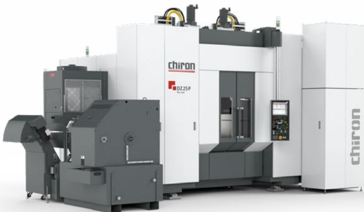
The double-spindle machining centre DZ 25 P five axis has been developed by CHIRON Group for highly productive machining of components with large-scale production. ©CHIRON
