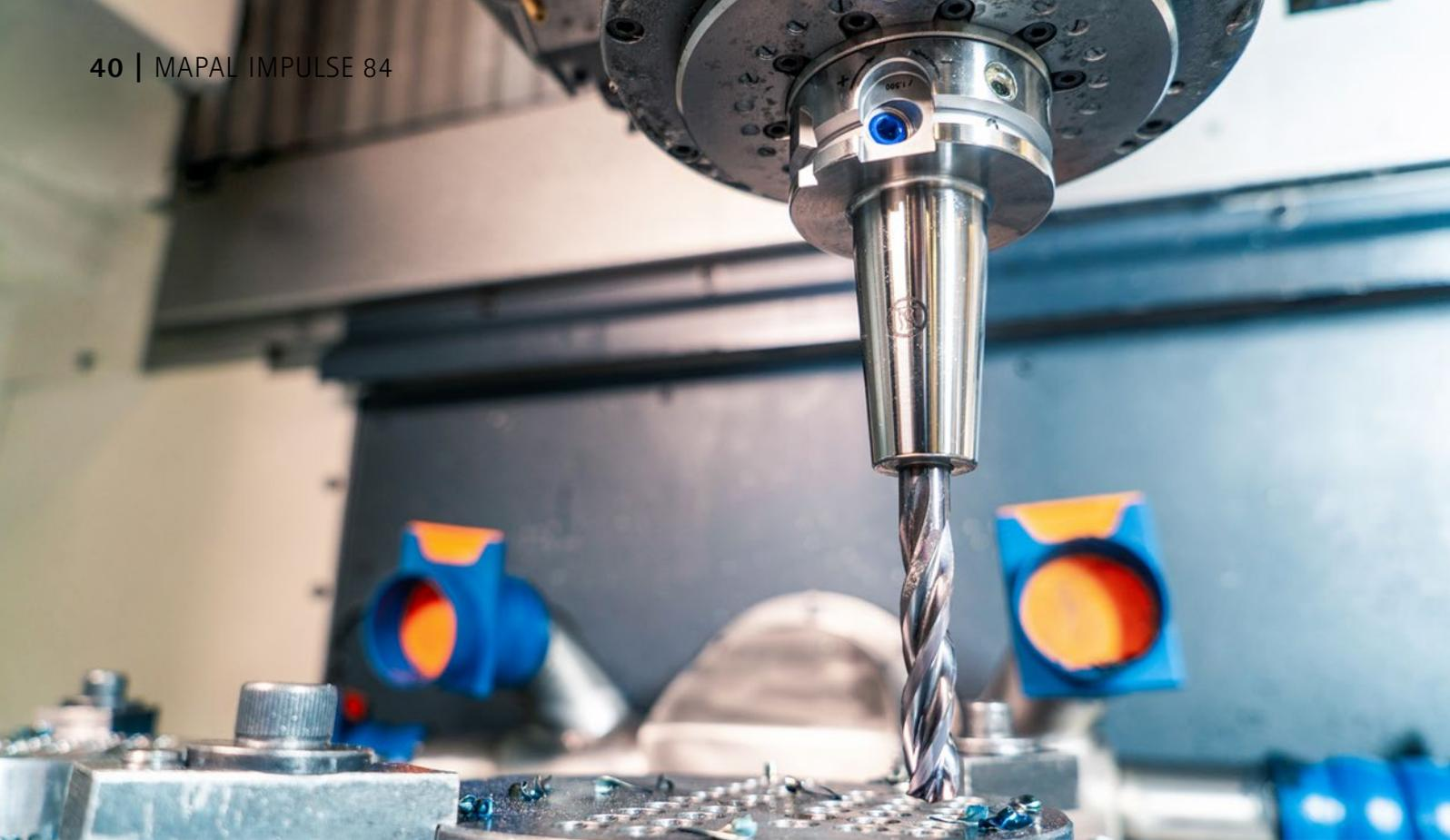
*A special design element on the UNIQ chuck is the blue actuating screw.*
