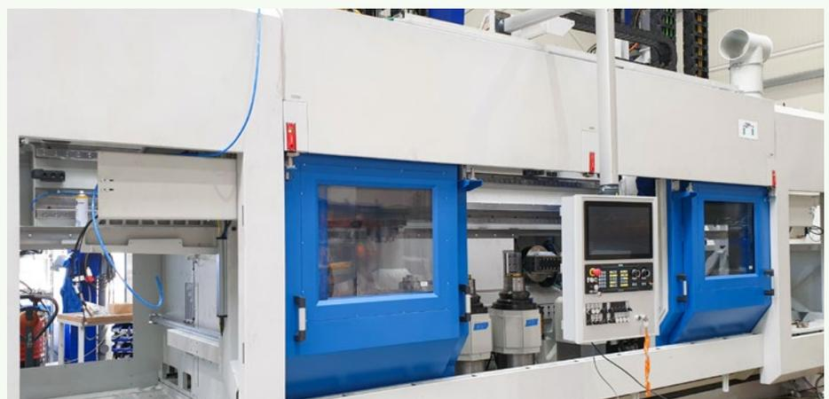
*At RASOMA, the next DZS 400-2 is currently being built. The pick-up area is on the left, the drop-down on the right. Various machining stations are set up between them.*
