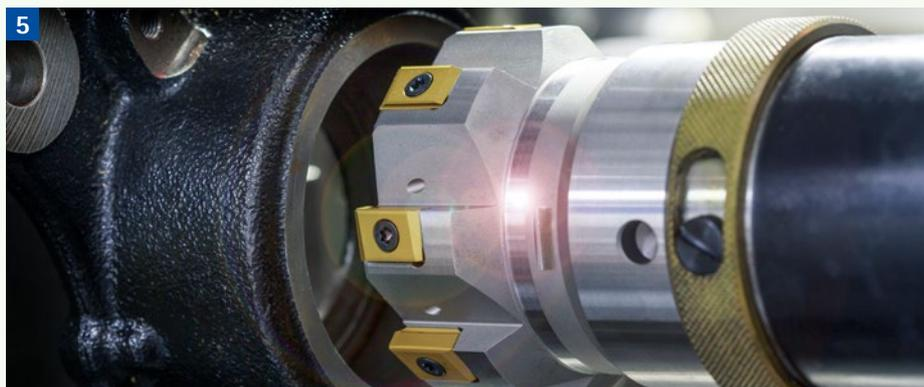
**5** HPR400 plus high-performance reamer for finish-machining the main bearing bore of a steel swivel bearing.
